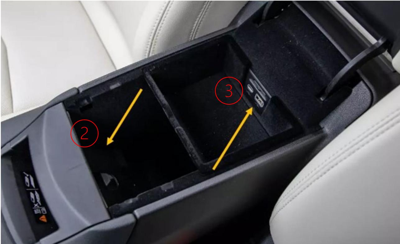
With the vehicle powered off, you can eject the existing SD Card from the slot by giving a gentle push on the SD Card and then pulling it out. ④
